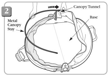
• Insert the metal canopy stay through the canopy tunnel.
